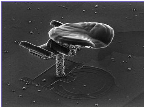
It takes some chops to build such a tiny Star Trek space craft, even though it does look a bit deflated from this angle. The two scientists used a focused ion beam to cut out this minuscule model, using a process called Chemical Vapor Deposition (CVD) that uses phenanthrene gas to etch the lit-
