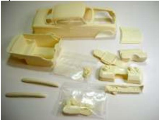
Almost all resin kits require a donor plastic kit for some of the parts. As you can see, this kit came with only the body and interior, no instructions, and very poorly cast parts. Since it came with an open hood, and the customer wanted it complete with an engine, using the chassis from the old Johan Lark kit wouldn't work.
