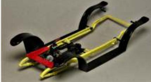
Chassis sub-assembly with engine/transmission installed
