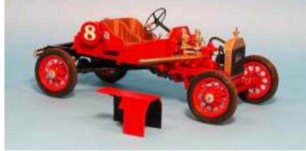
The engine is a modified Ford model T with dual carburetors and a custom open exhaust. I modified the Ford hood to clear the carburetors and exhaust. Wheels and tires are from a Monogram 1/24<sup>th</sup> scale Ford Model A kit.
