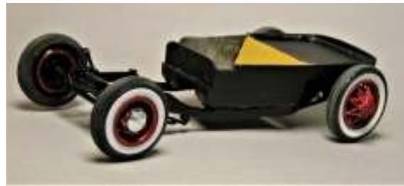
The rear axle and frame was Zee'D by cutting the assembly and moving it up into the body at the rear. I cut the interior tub off at the rear of the seat mounts, then fit that floor piece back into top of the rear of the interior. I scratch built a rear passenger compartment wall from .004" sheet lead. This turned the sedan into a two seat car.
