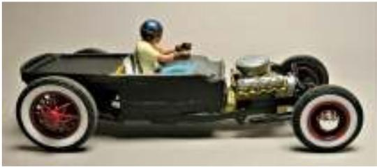
I turned the panel body into a Tudor sedan by removing the rear door. Since this was going to be a really low car, I added a Ross type steering box and steering gear from the cowl to the front pitman arm. I shortened the door height by re-scribing the lower edge and filled the old panel lines. I added a fuel filler and gas cap to the rear left quarter.
