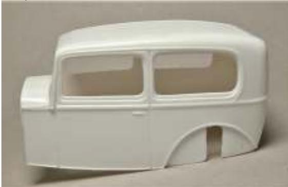
I was originally going to chop the top, but decided to leave it full height. Body has rear axle cutout for channeled body drop over frame rails. I moved the bottom of the doors up to clear the exhaust system and added Ross type steering gear.
