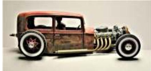
I added a scratch built pitman arm and drag link mounted on the outside of the cowl area. Other details were the gas filler tube and cap and Ramona sitting inside. I used the kit windows.
