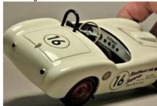
The Dash was made from sheet lead and the gauges are a decal I made for the project.
