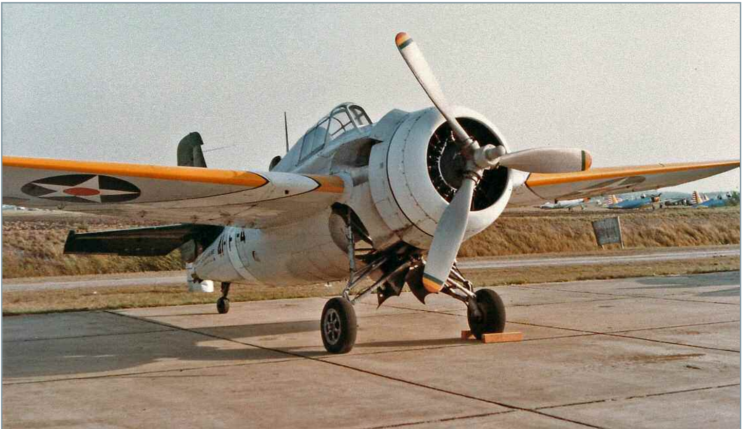
An FM2 Wildcat. It's painted as a prewar F4F, but the tall rudder gives it away.
