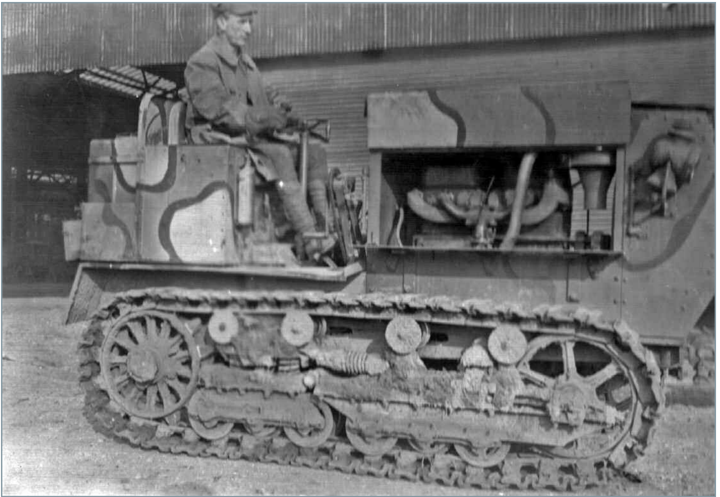
Here's a Holt artillery tractor; note the WWI camouflage—green, brown and yellow ochre with black outlines was a common scheme.
