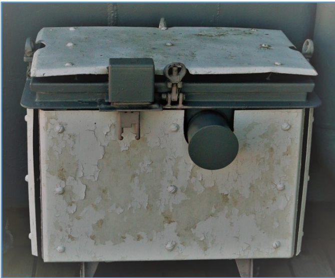
Pyrotechnic Locker hold various combustible items such as smoke grenades, flares, and ammunition for both machine guns and the saluting batteries
