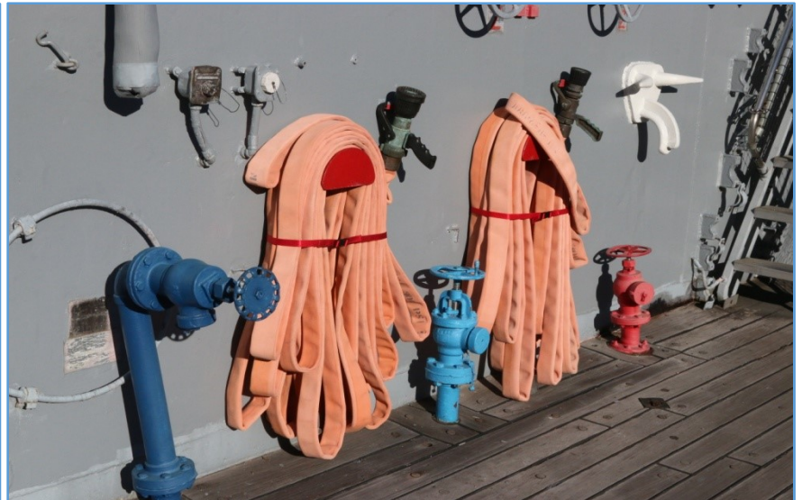
Every color has a specific safety meaning: Blue: fresh water, Green: salt water, Red/green stripe: fire fighting foam, White: steam, Gray: high pressure air, Tan: low pressure air, Orange: hydraulics, Yellow: fuel oil, Yellow and black: lube oil
