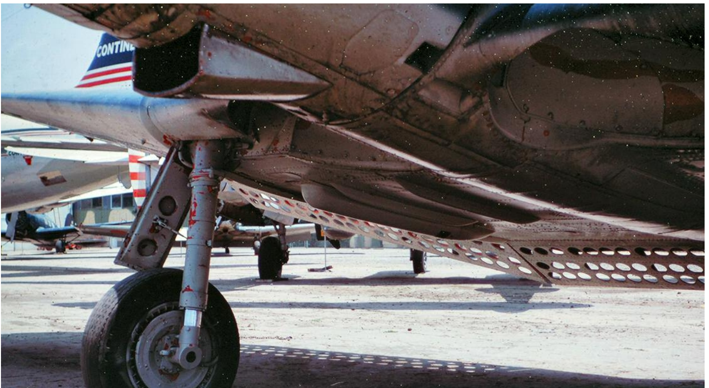
Wheel well and flap details on the SBD Dauntless shown in the December 2013 Newsletter.
