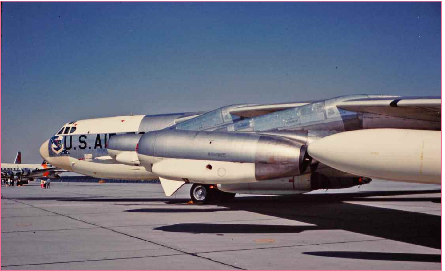
Below: This is the same B-52 with the missile, but I thought that the arc of the wing droop was interesting, so I took this photo to show the wing's flexibility.
