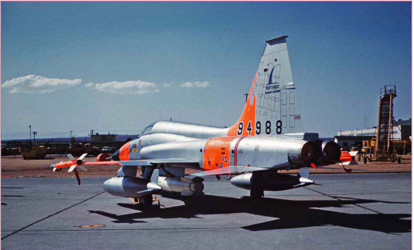
Air-to-air missiles on the wingtips of the second prototype YF-5A (Or is it already the F-5A?). The first prototype YF-5A was 94987, this airplane is 94988.
