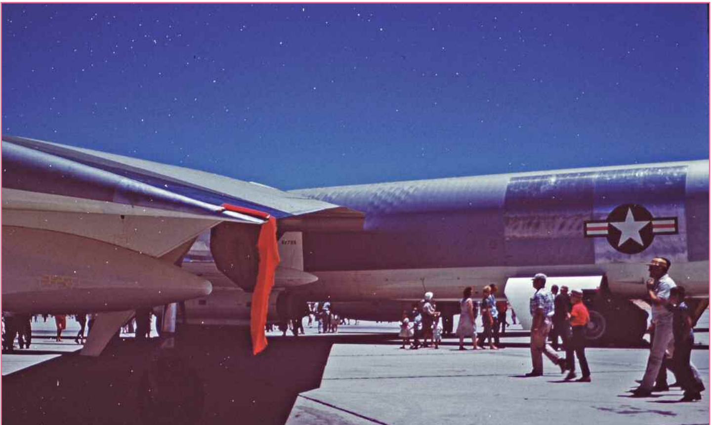
Below: This is the same B-52 with the missile, but I thought that the arc of the wing droop was interesting, so I took this photo to show the wing's flexibility.
