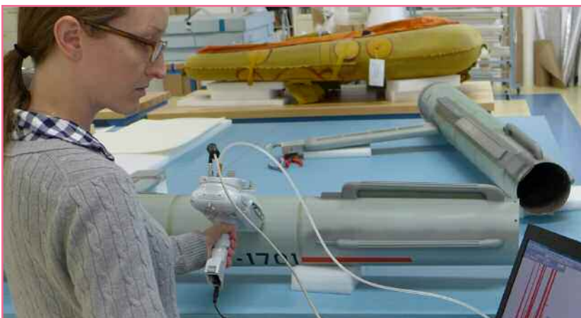
Above: A conservator conducts X-ray fluorescence spectrometry to determine the metal alloy used to construct the port nacelle.
