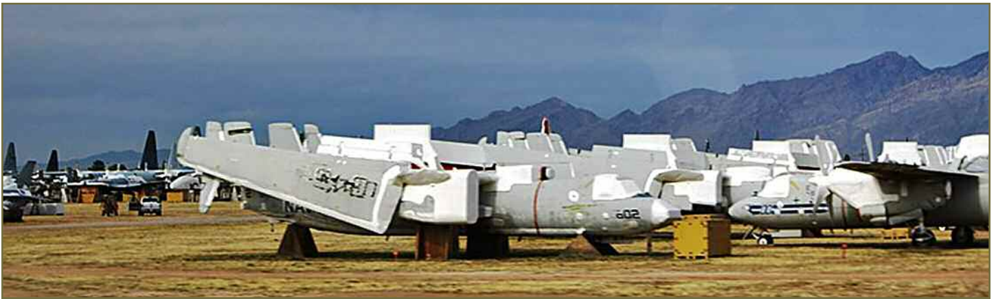
The Navy is not spared. These are earlier E-2Cs parked for parts. Looks like an E-2C from the VAW-77 Nightwolves waiting for its turn to be put on blocks. The first thing they remove on the Hawkeyes are the radomes because they produce an incredible amount of lift in the wind.
