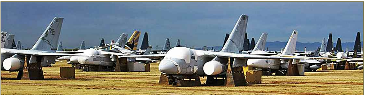
The Navy is not spared. These are earlier E-2Cs parked for parts. Looks like an E-2C from the VAW-77 Nightwolves waiting for its turn to be put on blocks. The first thing they remove on the Hawkeyes are the radomes because they produce an incredible amount of lift in the wind.
