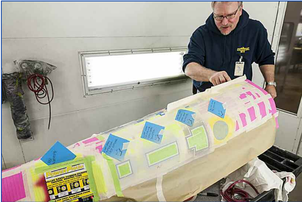
John Goodson shows off the complex masking used to create the markings on the bottom of the secondary hull of the Enterprise model.
