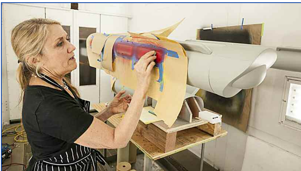
Kim Smith of Pulse Evolution adds red detailing to a carefully masked area of one of the Enterprise model's nacelles, or engine pods.
