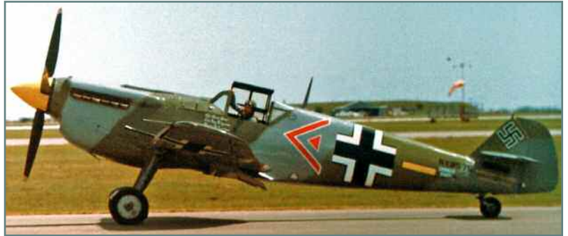
A former Spanish Air Force Hispano Aviacion HA-1112 M1L Buchon, a Bf-109 powered by a 1600 hp Rolls Royce engine.
