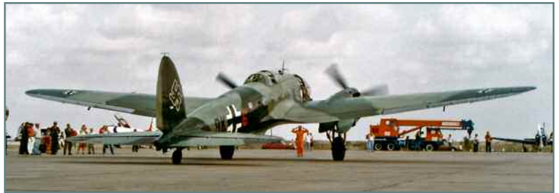
A CASA 2.111, a Heinkel He-111 powered by Rolls Royce Merlin engines. Formerly of the Spanish Air Force.
