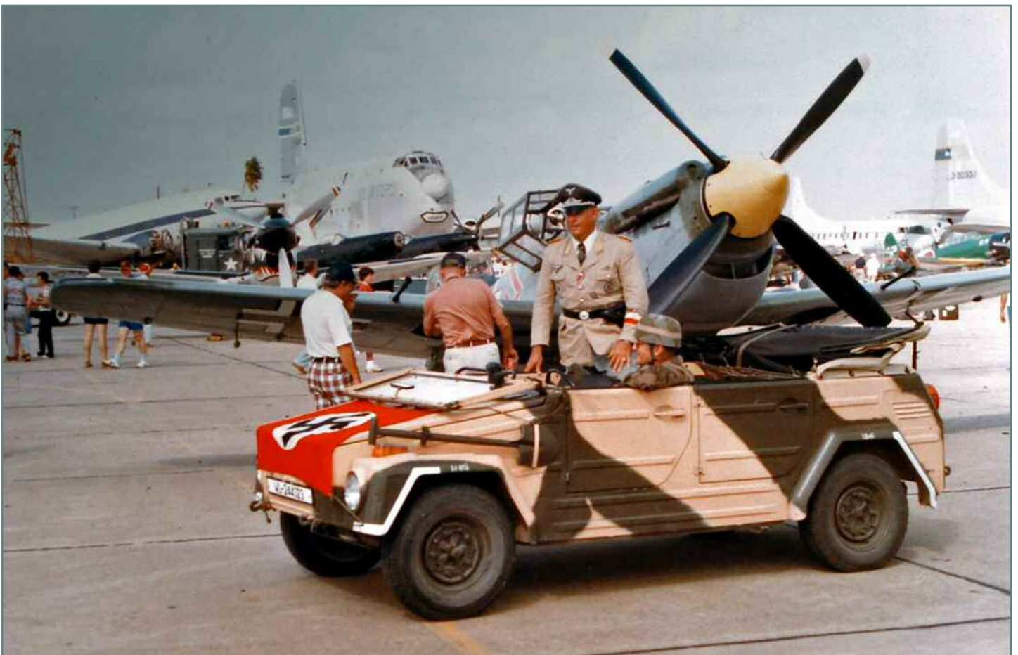
A Kubelwagen in front of the HA-1112 MiL Bf-109. Notice the aircraft's cowling and radiator shape, very different to the German Daimler Benz-powered airplanes.
