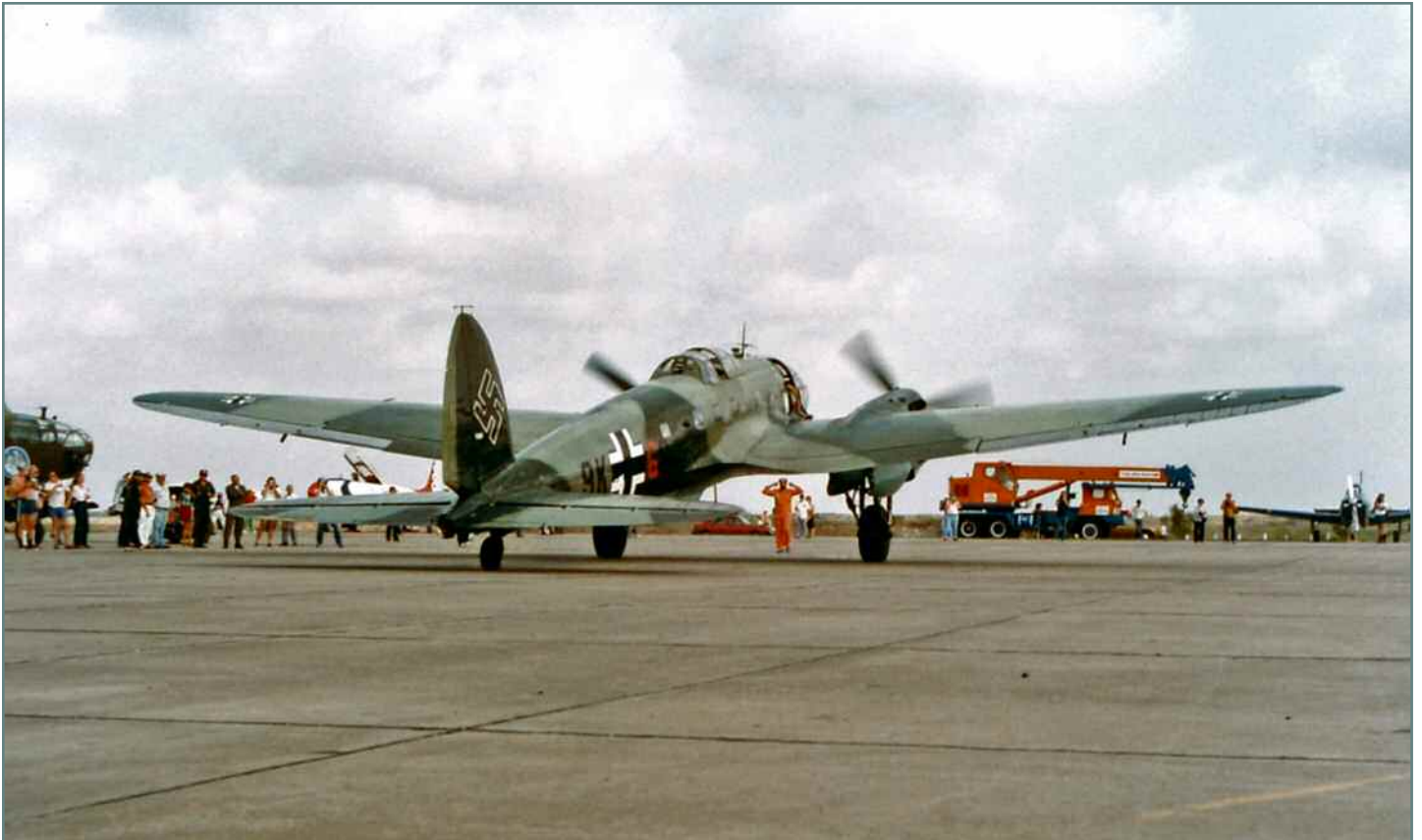
A CASA 2.111, a Heinkel He-111 powered by Rolls Royce Merlin engines. Formerly of the Spanish Air Force.
