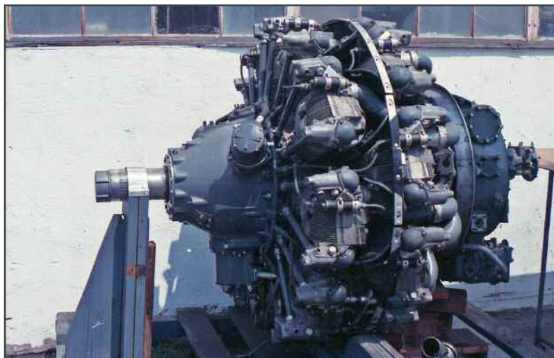
A double-row 18-cylinder radial engine on its stand. Not often can you view these engines outside their airplanes. This engine must have been a real bear to work on. I took these at the Planes of Fame museum at the Chino airport in September, 1988.
