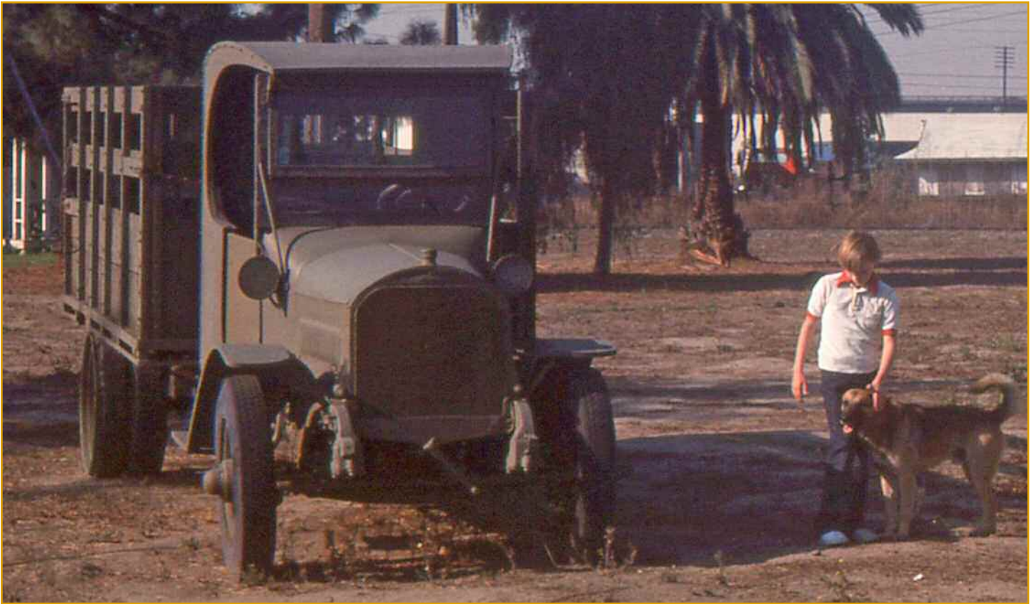
A World War I truck. Although it looks a bit primitive by World War II standards, it has dual rear wheels to provide better traction in the trench warfare conditions.
