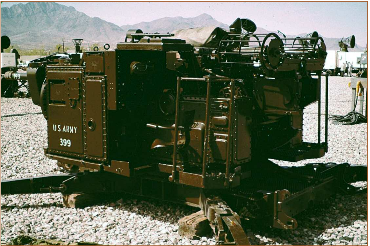
I think this is a Skysweeper, a radar controlled 75mm anti-aircraft gun. Renwal had a model of this gun in the 1960s.
