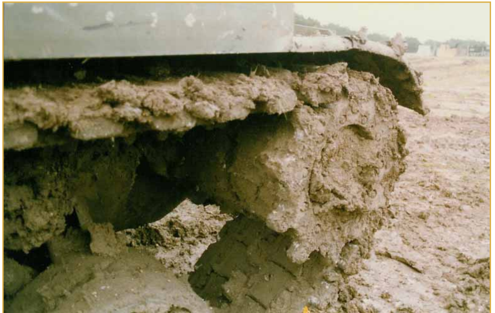
It can clog up tracks, wheels, and drive sprockets.
