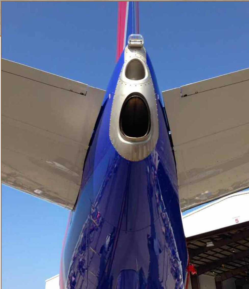
Left: The aft section, with light, APU exhaust, and other details.
