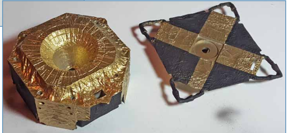
Masking and painting the black over the gold on the lower LM section.
