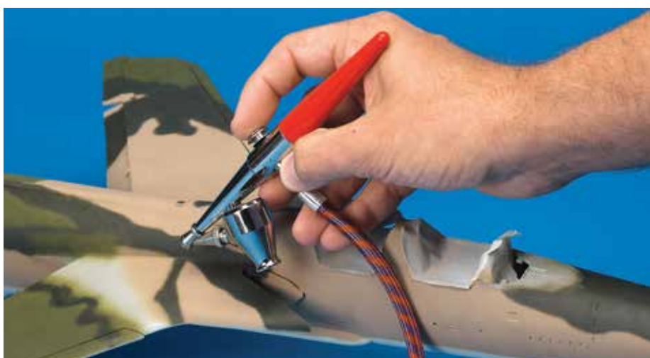
Spray cans are all right for some jobs, but complex camouflage is not one of them. An airbrush gives you the versatility you need for a wide range of paint effects.
