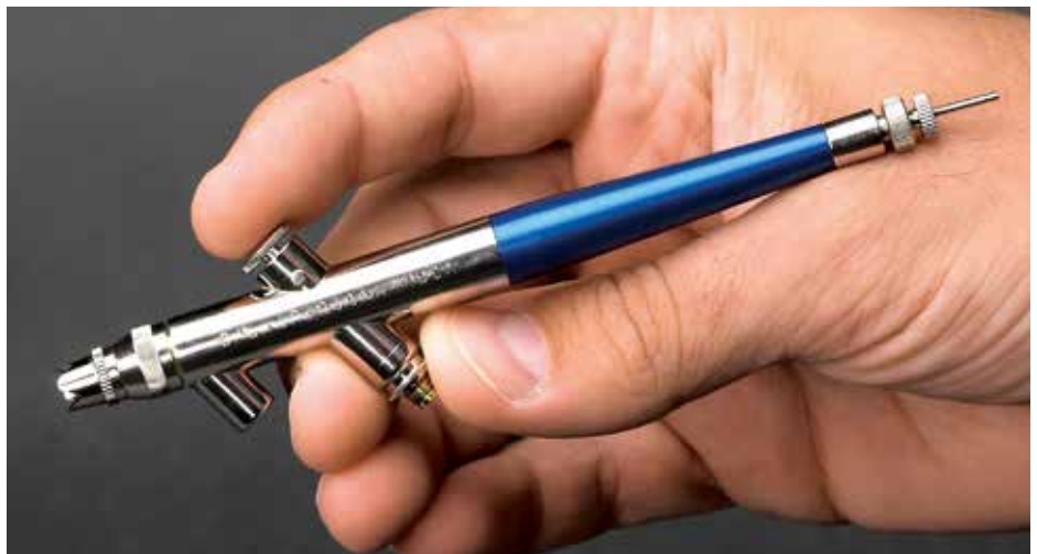
Single-action brushes: An external-mix airbrush (black) brings paint from the outside to the tip; the internal-mix airbrush draws paint inside the airbrush and through to the tip. The latter must be disassembled to be cleaned, but provides finer atomization of the paint. The thumbscrew at the back end sets paint volume; the pushbutton controls air pressure.
