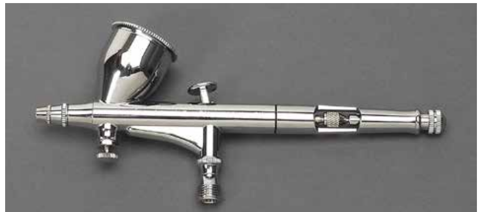
This double-action airbrush has all the bells and whistles a modeler could want: gravity-feed paint cup; the thumbscrew below the cup sets a baseline air pressure; the pushbutton trigger behind the cup controls both paint volume and air pressure; and the thumbscrews behind that regulate paint volume, too.
