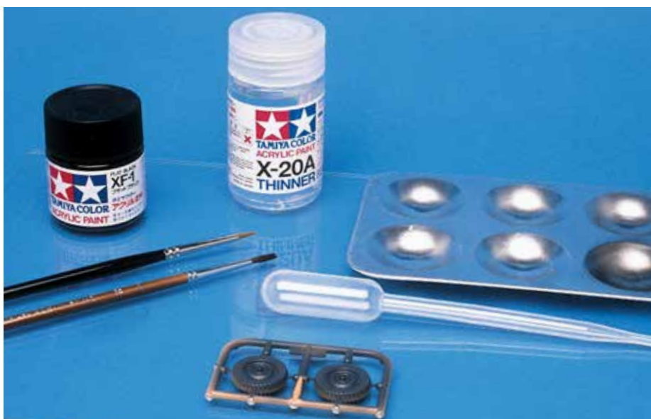
Tamiya paint, Tamiya thinner: Using the same brands guarantees compatibility. Mix the paint thoroughly, then use the dropper — not the brush — to extract clean, chunk-free paint from the jar. Put a little thinner next to the paint on the palette.
