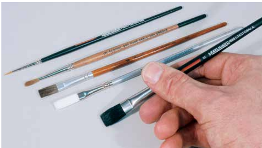
From the top: Testors Model Master No. 0 synthetic; Floquil No. 3 round pure sable; Floquil 1/4" flat Silver Fox synthetic; and Testors Model Master 1/2" flat black sable.
