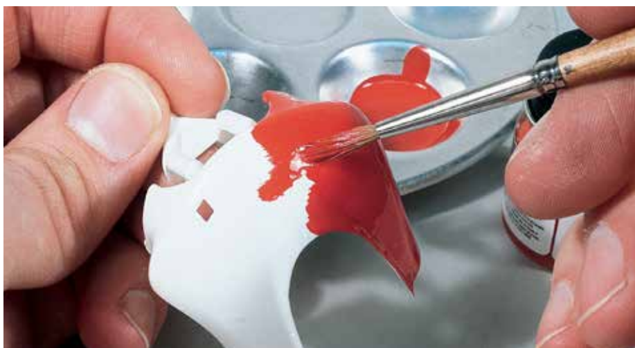
Use as few strokes as possible; begin in a bare area and work back to the wet paint. Keeping a "wet edge" prevents going over drying paint and minimizes brush marks.
