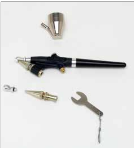
Single-action brushes: An external-mix airbrush (black) brings paint from the outside to the tip; the internal-mix airbrush draws paint inside the airbrush and through to the tip. The latter must be disassembled to be cleaned, but provides finer atomization of the paint. The thumbscrew at the back end sets paint volume; the pushbutton controls air pressure.
