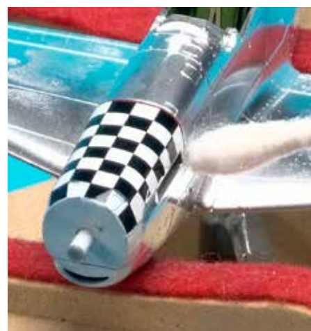
You can save cleanup time by soaking up excess water and decal setting solution right away with a cotton swab. But if there is solvent on the decal, put the swab down and back away from the workbench. After applying decal solvent, never touch the decal until it is dry.
